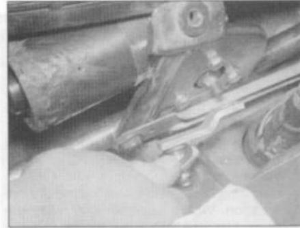
13.8 Unscrew the nut securing the linkage drive arm to the motor spindle
