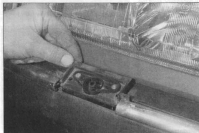
15.27b ... then prise out the feed tube assembly ...
