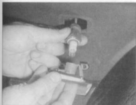
5.24b ... then twist the bulbholder anti-clockwise
