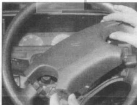
21.5 ... then ease the airbag unit from the steering wheel ...
