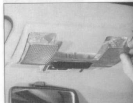
6.2 Prise the lens from the courtesy light ...
