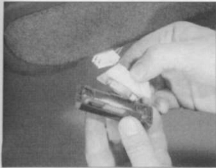
6.8 Unclipping the lens from the kerb light
