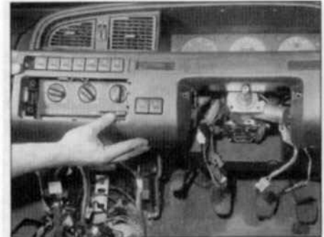
9.12 Withdraw the switch/heater control/display trim panel
