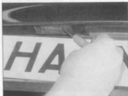
5.44a Prise the lens from the number plate light unit ...
