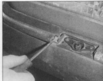
15.27a Unscrew the two feed tube securing screws ...
