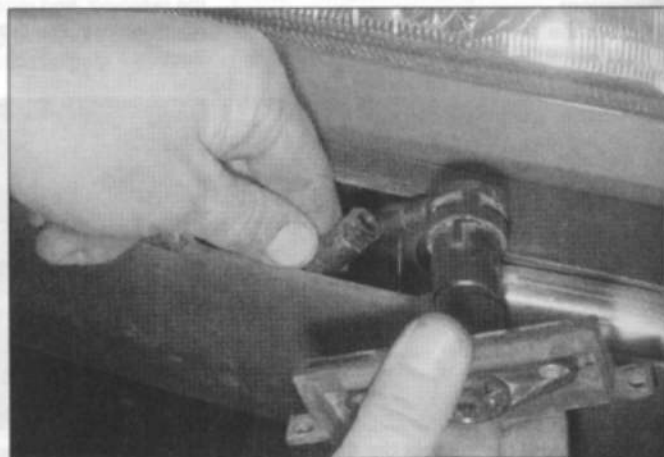
15.27c ... and disconnect the washer fluid hose
