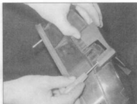
7.15 Unclipping a trim panel from a rear wing-mounted rear light - Hatchback model
