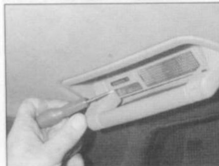
6.5 Prise the rear courtesy light assembly from the roof ...
