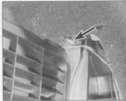
7.14a Unscrew the rear wing-mounted light upper securing nut ...
