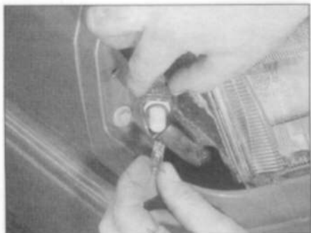
5.11 The bulb is a push-fit in the bulbholder
