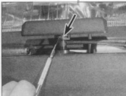
15.26 Prise the headlight washer nozzle from the bumper, and prise off the circlip (arrowed)
