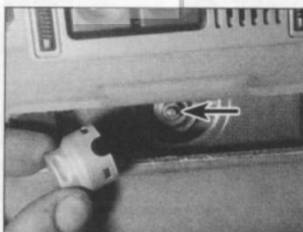
18.2 Prise the cover from the bottom of the aerial to expose the securing nut (arrowed)
