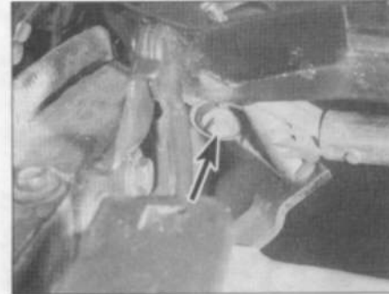
13.5b Wiper linkage-to-scuttle securing bolt (arrowed)
