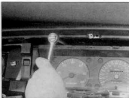
9.17 Unscrewing an instrument panel upper securing nut
