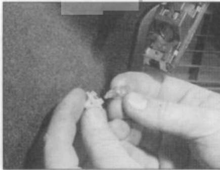
6.11 The luggage compartment light bulb is a push-fit in the bulbholder – Hatchback models
