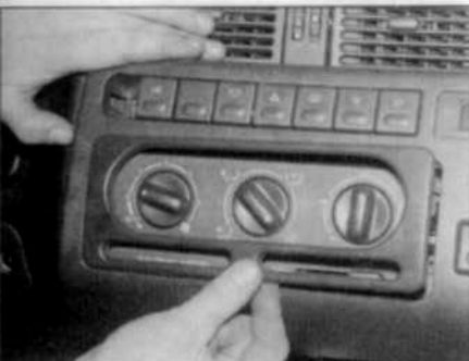
9.10a Prise out the heater control surround panel ...
