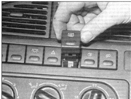
4.9 Removing a facia-mounted switch
