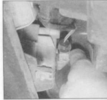
5.14 Twist the direction indicator bulbholder anti-clockwise
