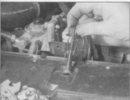
7.4 Pull out the headlight adjuster knobs
