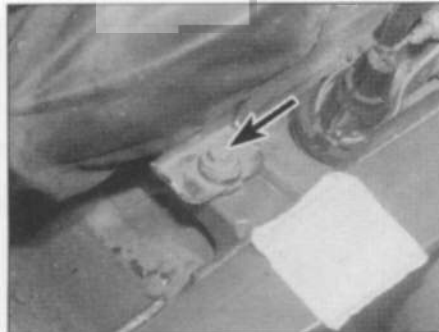
13.5a Unscrew bolt (arrowed) securing the wiper motor bracket
