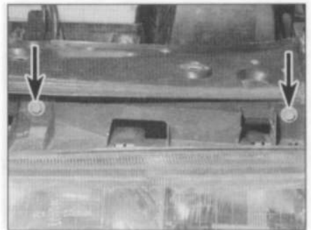
7.6a Unscrew the upper headlight securing bolts (arrowed) ...
