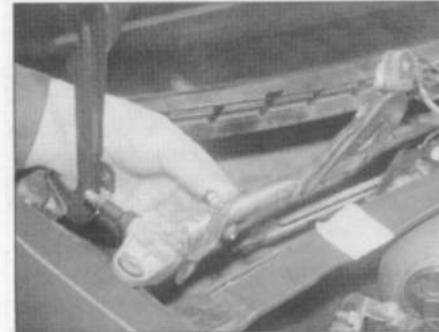
13.10 Manipulate the linkage out from the scuttle
