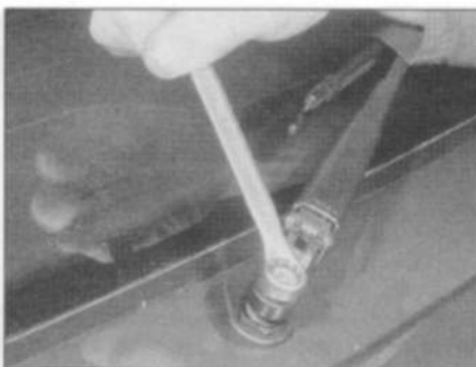
12.3 Unscrew the wiper arm spindle nut ...
