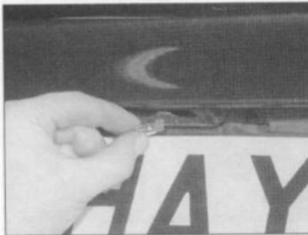
5.44b ... then pull out the bulb - Hatchback models
