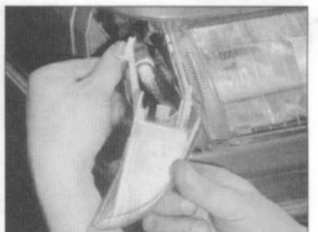
5.9b ... then push the sidelight assembly from the wing panel
