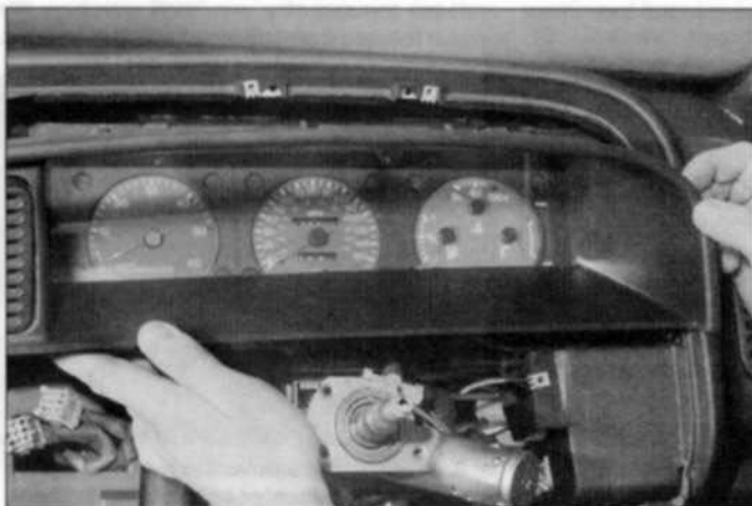
9.15 Withdrawing the instrument panel shroud
