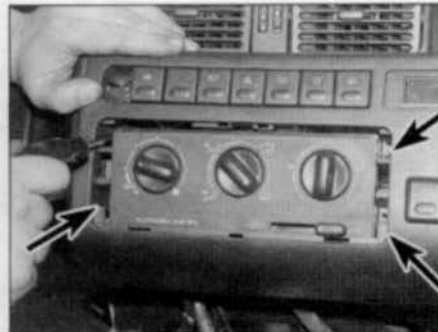
9.10b ... then unscrew the four heater control panel securing screws (arrowed)
