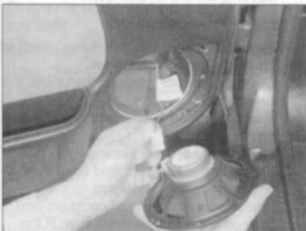
17.6b ... then remove the screws and withdraw the loudspeaker
