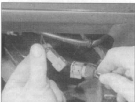
6.5b . . . and disconnect the foglight wiring connector
