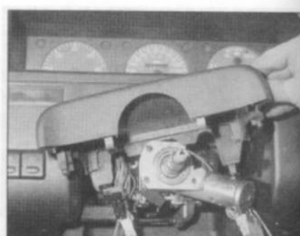
23.23 Removing the upper steering column shroud - models from 1995
