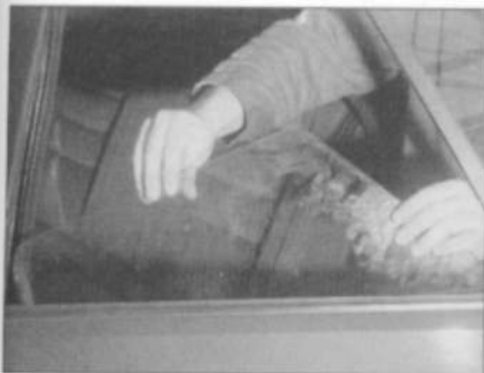
12.15 Withdrawing the rear door window glass
