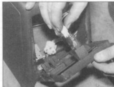
24.11 Unclip the rear ashtray surround and disconnect the wiring
