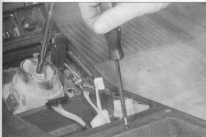
24.10a Unscrew the securing screws . . .
