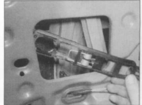
11.6c ... and withdraw the inner part of the handle
