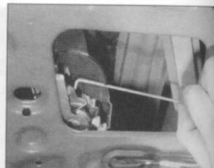
11.17a . . . then disconnect the operating rods . . .
