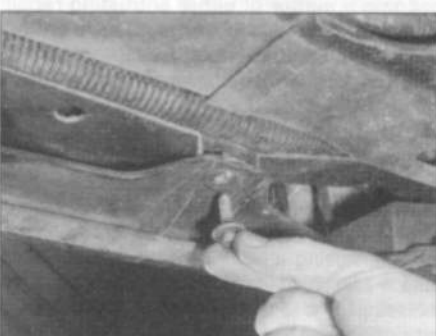
6.9a Unscrew the lower bumper securing screws . . .
