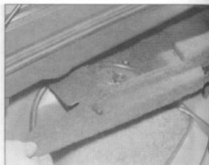
23.38c ... and lift out the parcel shelf side support panel
