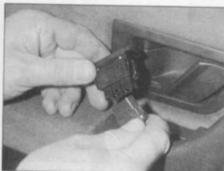
10.5 Removing the electric window control switch – front door
