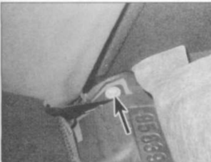
21.12 Fold the seat back down for access to the remaining seat back hinge bolts (arrowed) – Hatchback model
