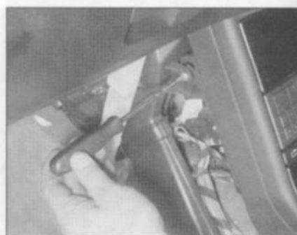
24.4 Unscrewing a heater duct securing screw
