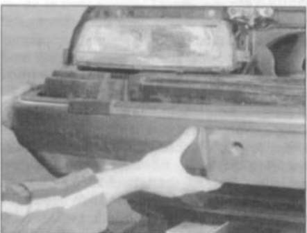
6.9b . . . and withdraw the bumper
