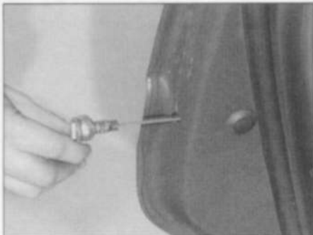
11.8 Unscrewing the rear door handle plastic block securing screw
