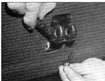
22.11 Pull off the circlip, and pull out the seat belt pivot pin ...
