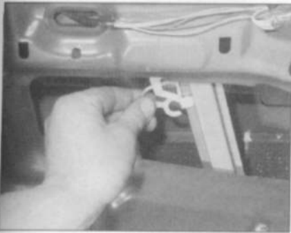
12.5a Pull off the plastic clip securing the window glass to the regulator – front door
