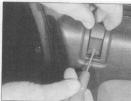
10.2 Depress the retaining tab and slide off the lock operating button
