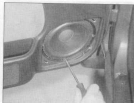
10.4 Unscrewing a loudspeaker securing screw – front door
