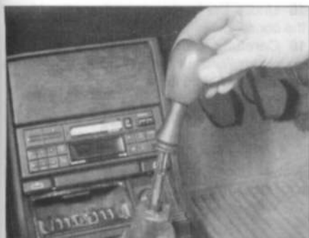
24.5 Pulling off the gear lever selector knob
