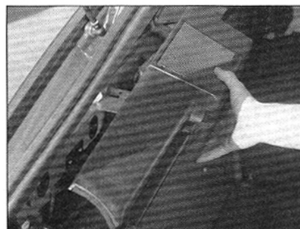
22.21 Removing the parcel shelf support panel - Estate model
