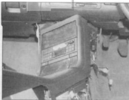
24.18 Withdrawing the centre console
