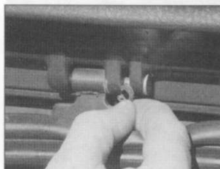
13.12 Prising the locking clip from a tailgate hinge pin – Estate model
