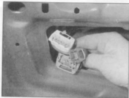
11.15 Disconnect the wiring plugs from the door lock assembly
