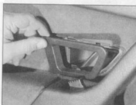
10.6 Unclip the surround from the door interior handle – front door
