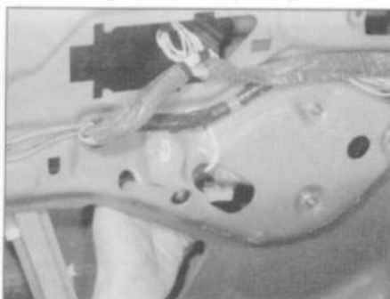
12.18 Disconnecting the front door window regulator motor wiring plug
