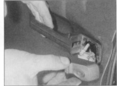
11.10b ... then pull the lock cylinder assembly from the exterior handle
