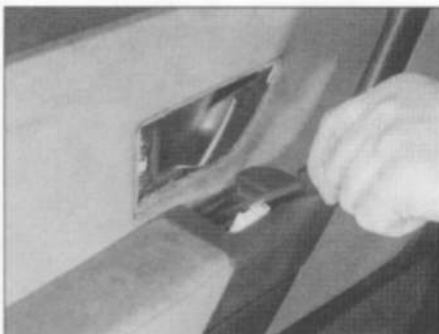
10.11 Unscrewing the door trim panel securing screw from the electric window switch aperture – rear door
