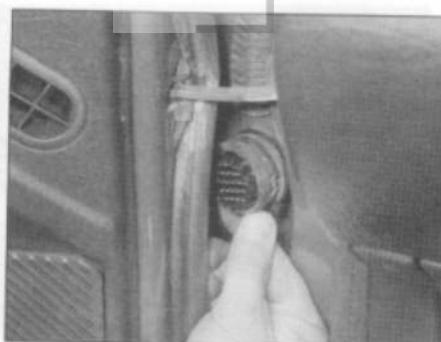
9.2 Disconnect the door wiring connector
