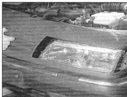
20.4c . . . and withdraw the front grille panel
