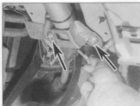
13.11 Removing the steering column universal joint clamp bolt – lower steering column securing nuts arrowed
