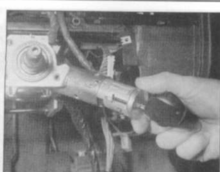
14.7b . . . then pull the lock cylinder from the housing
