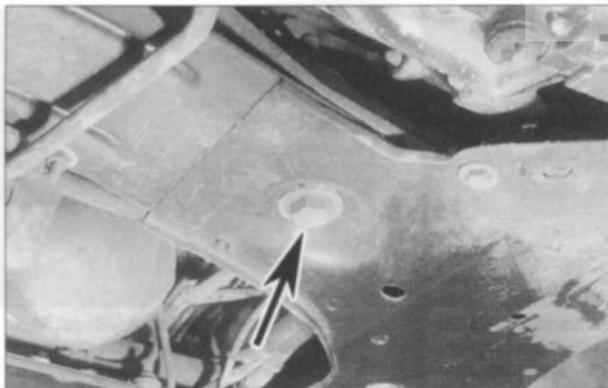
15.12 Steering gear securing bolt (arrowed)
