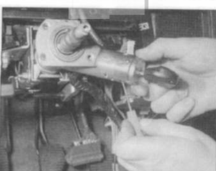
14.7a Depress the lock securing lug . . .
