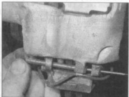
4.4b ... then remove the caliper retaining pin
