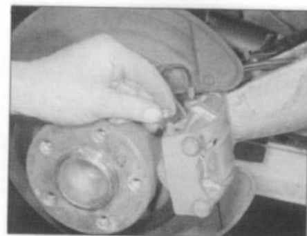
2.13b Removing the dust cap from a rear caliper bleed screw
