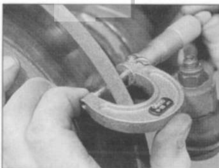
6.3 Using a micrometer to measure disc thickness
