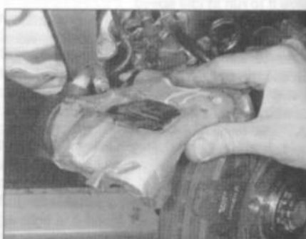
4.6 ... and swivel the caliper upwards
