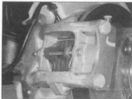
5.11 View of caliper showing anti-rattle spring and pad retaining pin correctly fitted
