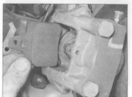
5.4 Sliding the inboard pad from the caliper
