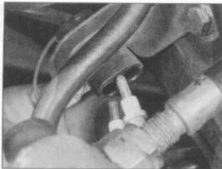
4.2 Disconnecting the brake pad wear sensor wiring connectors
