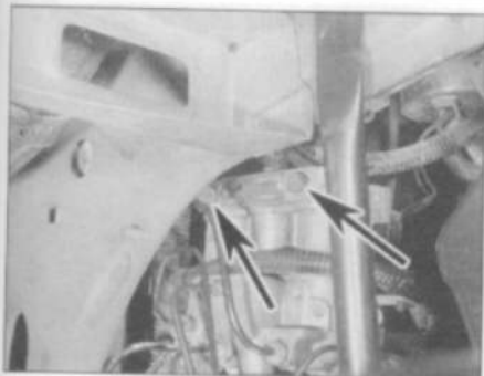
2.8 ABS hydraulic valve block bleed screws (arrowed)
