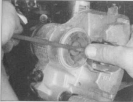
4.11 Using a length of flat bar to retract the caliper piston
