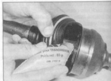
4.11f Pack the joint with the grease, working it into the ball tracks while twisting the joint, then locate the gaiter outer lip in its groove on the outer member
