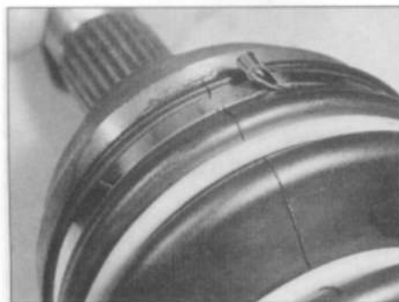
4.11i Fold the clip end underneath the buckle ...
