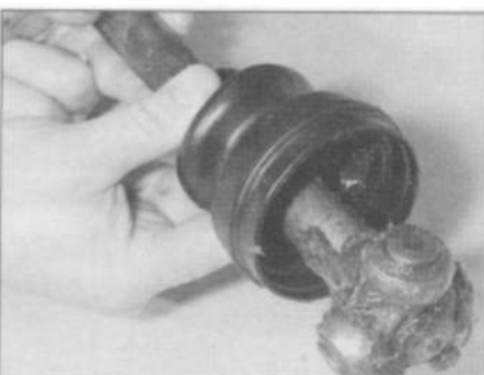
3.7b Slide the gaiter off the end of the driveshaft . . .
