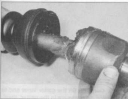
3.7a Release the inner gaiter retaining clips, and remove the joint outer member
