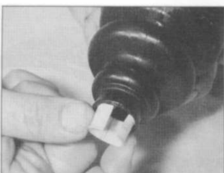
3.7c . . . and remove the plastic bush
