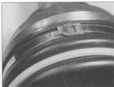
4.11j ... then fold the buckle firmly down onto the clip to secure the clip in position
