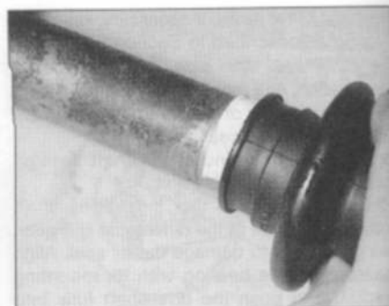
4.11c ... and seat the gaiter inner end on top of the plastic bush
