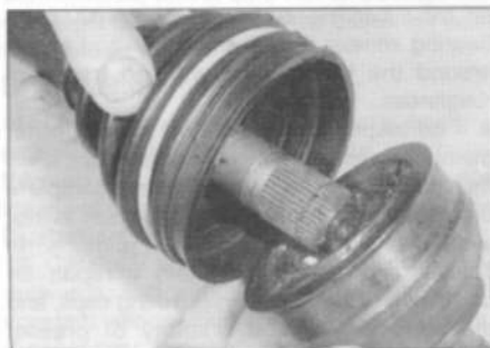
4.11e ... then locate the joint outer member on the splines, and slide it into position over the circlip. Ensure that the joint is retained by the circlip before proceeding
