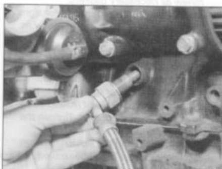
5.29b Unscrew the oil supply line union at the cylinder block ...
