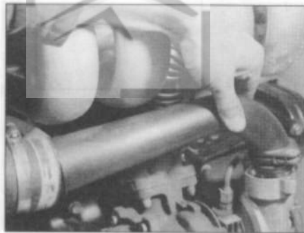
5.23a Disconnect the air ducting from the ports on the turbocharger...
