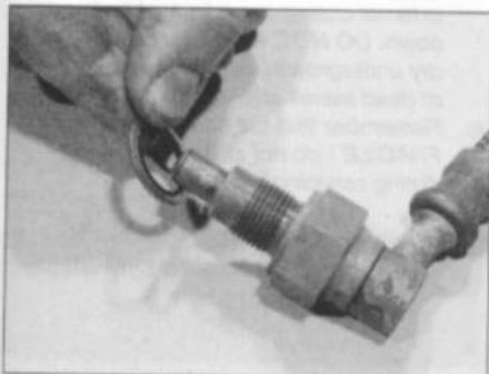
5.29a Renew all gaskets and oil supply and return union seals
