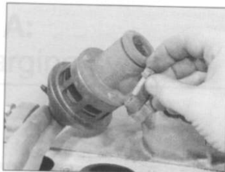
10.11 Remove the screws and lift the EGR valve from the manifold - 2.5 litre model shown
