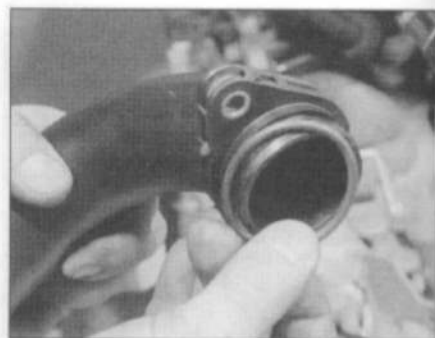
5.23b ... and recover the O-ring seals - 2.5 litre model shown
