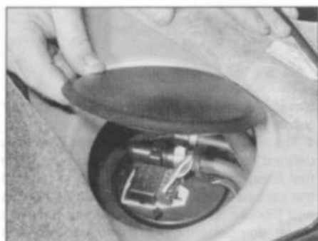
8.3a Remove the plastic cover . . .
