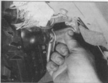
9.38 ... then pull the pipes from the matrix
