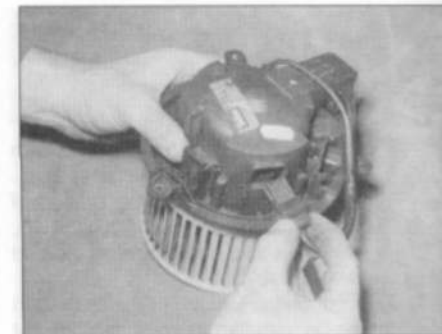
9.26a Pull the motor wiring plug out of the housing ...
