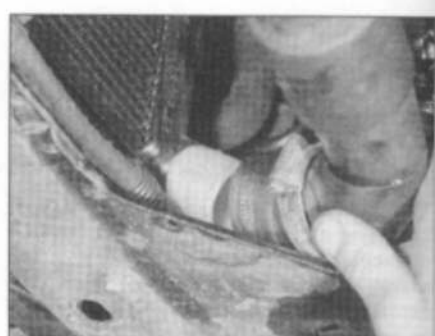
3.4a Disconnecting the lower radiator hose
