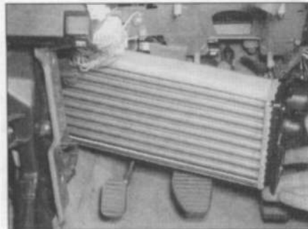
9.44 ... then slide the new matrix into the housing
