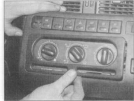
9.17a Prise out the heater control surround panel ...
