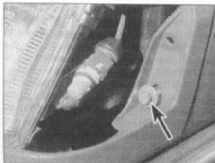
3.3a Unscrew the front grille panel securing bolts (arrowed) from the sidelight apertures ...
