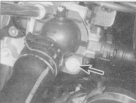
4.6 Unscrew the thermostat cover bolts ...
