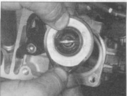
4.7 ... and lift out the thermostat and sealing ring – petrol engine
