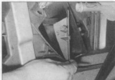
9.42a Cut away the front corner of the heater matrix housing ...
