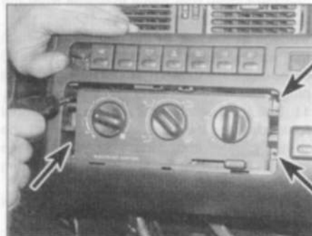
9.17b ... then unscrew the four heater control panel securing screws (arrowed)
