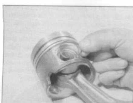
15.19c . . . then fit two new circlips
