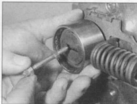
8.4b . . . then unscrew and remove the stud
