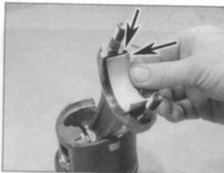
21.5a Press the bearing shells into the connecting rod ...
