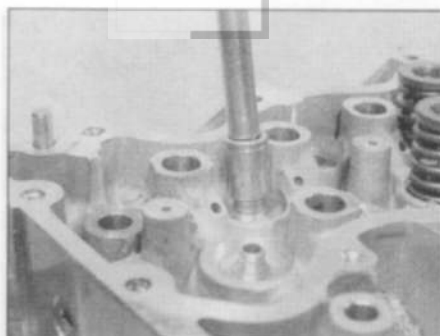
10.2b Use a suitable socket or metal tube to press the seal firmly onto the guide
