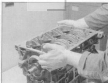
20.30b Lower the bearing ladder into position over the crankshaft
