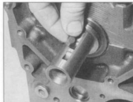
13.5c Remove the Woodruff key, and store it with the sprocket for safe-keeping
