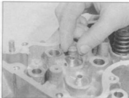
10.2a Carefully locate the new valve stem oil seal over the valve and onto the guide
