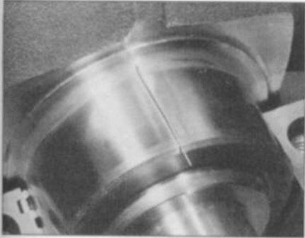
20.17 Plastigauge in place on a crankshaft main bearing journal
