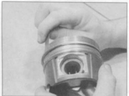
15.2 Using an old feeler blade to aid the removal of the piston rings
