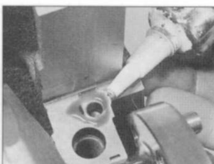
20.39 Apply a small amount of sealant to the No 1 main bearing cap mating face on the cylinder block, around the sealing strip holes
