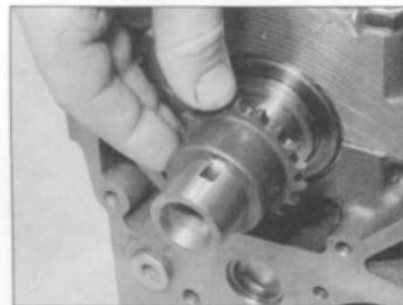
13.5b . . . and slide the drive sprocket and spacer (where fitted) off the end of the crankshaft
