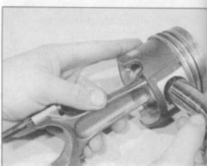
15.15b ... and push out the gudgeon pin - 2.1 litre model shown
