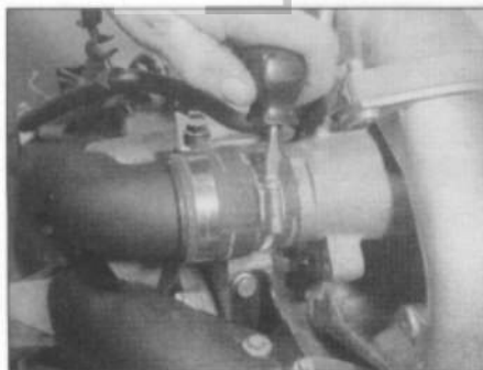
6.33b On 2.5 litre models, slacken the hose clips ...
