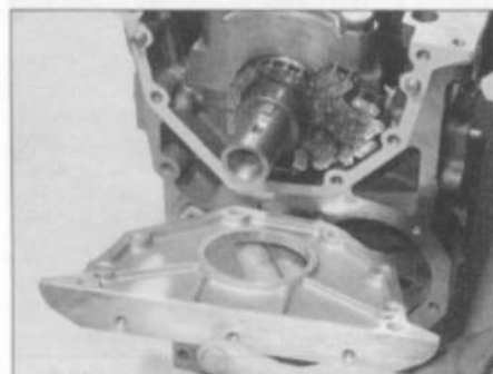
13.4 Remove the oil seal carrier from the front (timing belt) end of the cylinder block - XU and XUD engines
