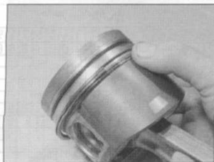
19.10b ... then the oil control ring
