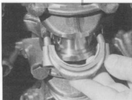
12.5 Removing a big-end bearing cap and shell
