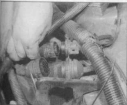
6.19 Unplug the main engine wiring harness at the connectors, located above the transmission casing
