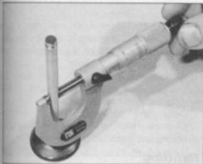
9.12 Measure the valve stem diameter at several points using a micrometer
