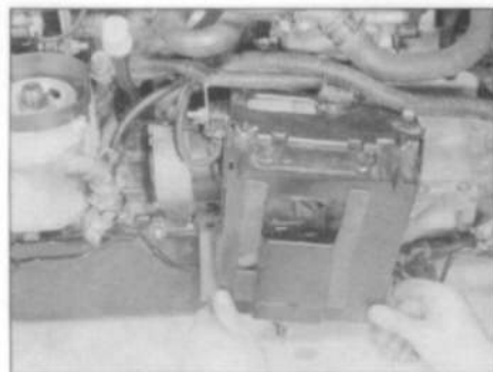
6.33a On 2.5 litre models, unbolt the intercooler mounting bracket from the engine block
