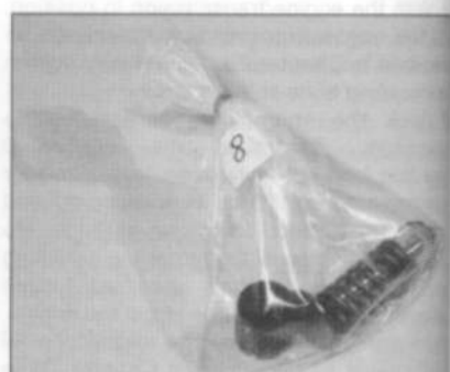
8.9 Keep each valve and its associated components together in a labelled bag
