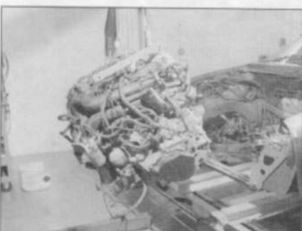
6.30 Lift the engine and transmission assembly out over the front crossmember
