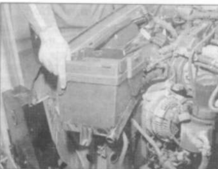
6.13 Remove the electronic control units from their plastic casing, then remove the casing from the bodywork
