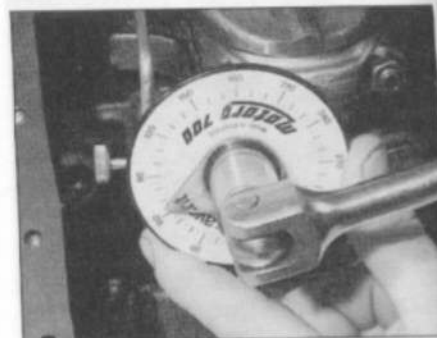
21.22b ... then angle-tighten them through the specified stage 2 angle, using a socket and extension bar
