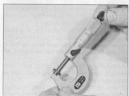
11.14b Using a micrometer to measure shim thickness
