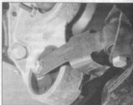
18.24 Rear engine mounting and link
