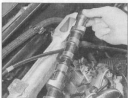
10.9 . . . then lift the camshaft away from the cylinder head
