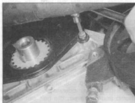
6.4b Unscrew the retaining bolts ...
