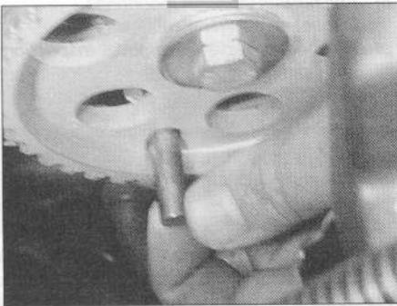
3.7 9.5 mm diameter drill inserted through the camshaft pulley timing hole
