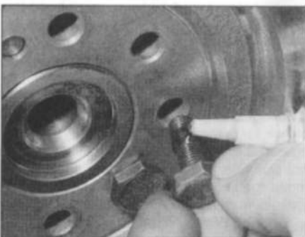
17.10 If the new flywheel bolt threads are not supplied with their threads pre-coated, apply a suitable locking compound . . .
