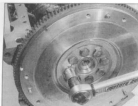
17.12 ... then refit the flywheel, and tighten the bolts to the specified torque
