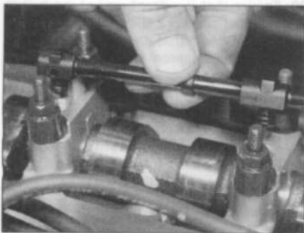
10.5 Removing the oil supply pipe from the camshaft bearing caps
