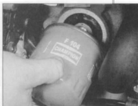
3.8b . . . then unscrew it by hand the rest of the way
