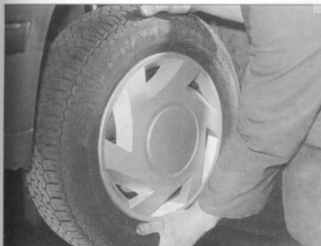
7.4 Check for wear in the hub bearings by grasping the wheel and trying to rock it
