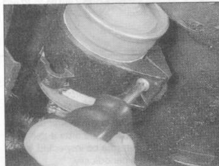
17.3 Unscrew the screw and release the filter retaining clamp
